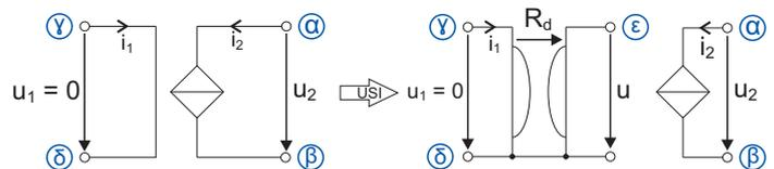
$i_2 = \beta \cdot i_1 \quad u = R_d \cdot i_1 \quad i_2 = \frac{\beta \cdot u}{R_d}$
