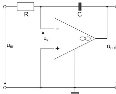
$u_{out} = -u_c(t_0) - \frac{1}{RC} \cdot \int_{t_0}^{t_1} u_{in} dt$
