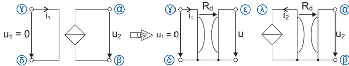
$$u_2 = \beta \cdot i_1 \quad u = R_d \cdot i_1 \quad i_2 = \frac{u}{R_d} \quad u_2 = -R_d \cdot i_1$$
