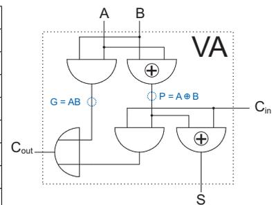
$$S = P \oplus C_{in}, \quad C_{out} = G + P \cdot C_{in}$$
